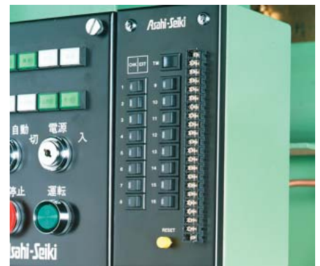
■ Workpiece transfer detecting device is to detect mis-transfer of workpieces between the stations to stop the machine and avoid tool breakage.
