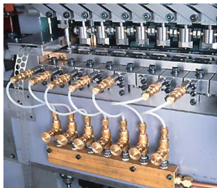
■ Oil lubrication device is to supply drawing oils by compressed air from reservoir into dies to lubricate material during drawing operation.
